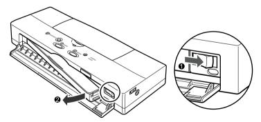
**5.** Remove the battery pack from the printer.
